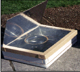
Figure-8: Box type solar cooker
